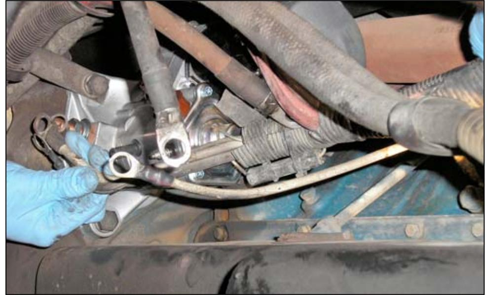
**Remove the tie holding the battery cable.**
