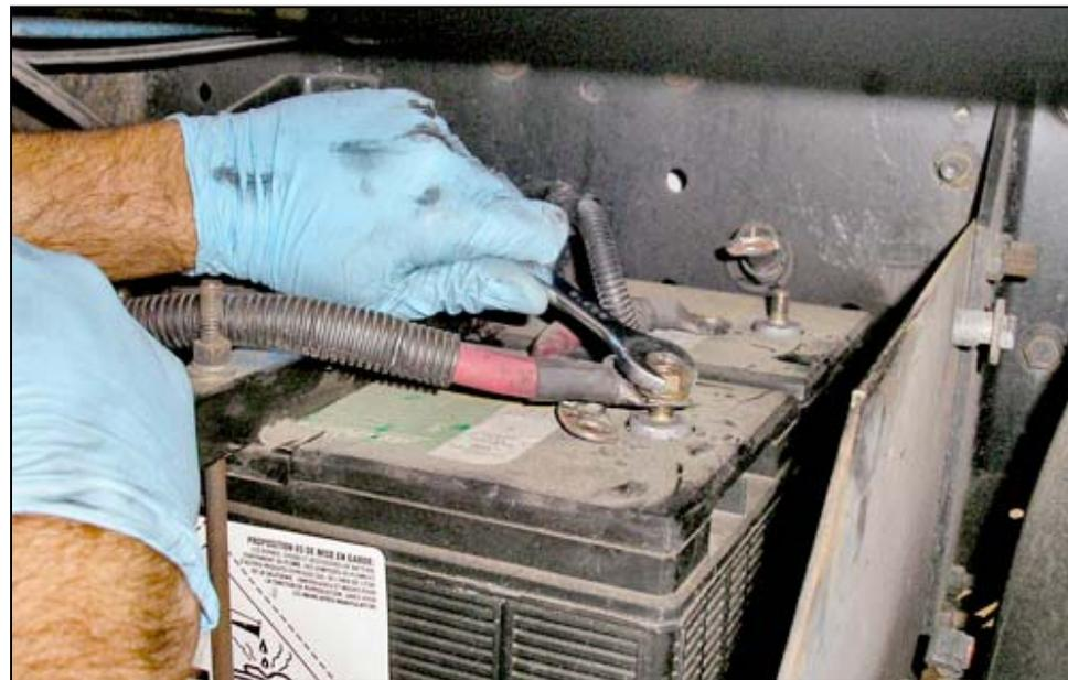
**Check the voltage of all batteries. Each battery should be fully charged.**
