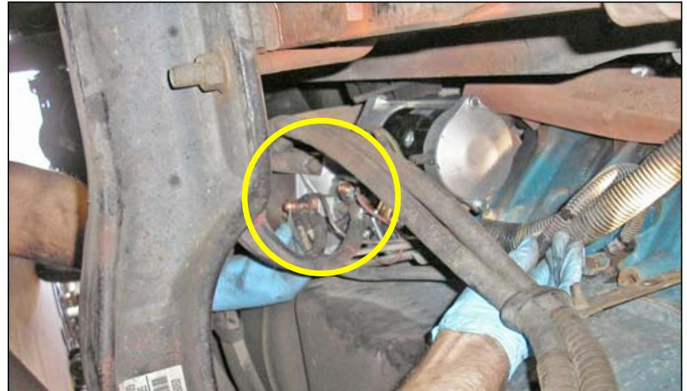
**Secure all ground cables to the negative (-) terminal (Terminal G) with retaining nut.**
