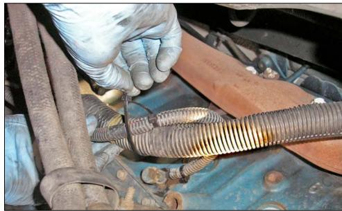
Locate the 50 terminal (key switch) stud on the starter.
