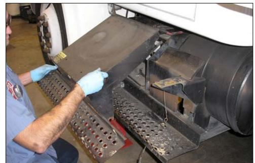
Disconnect and isolate the negative (-) battery cable from the negative (-) battery terminal.
