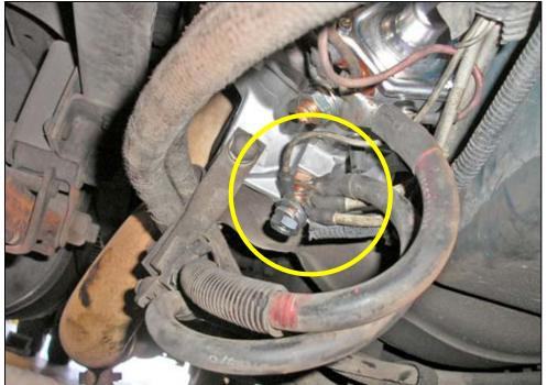
Tighten and torque the Terminal G retaining nut to:
