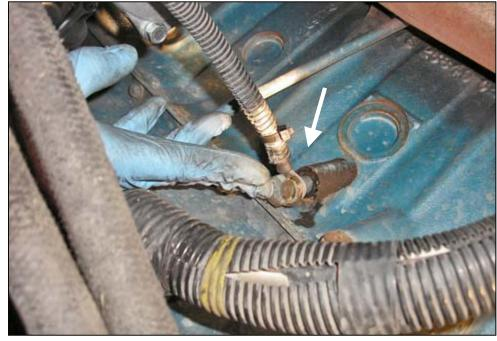
Secure the opposite end of the engine block ground cable to the negative (-) terminal (Terminal G) of the starter.
