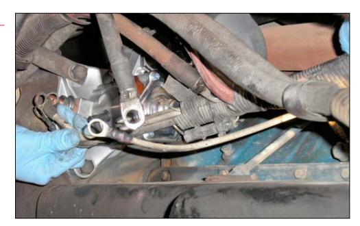
Remove the tie holding the battery cable.
