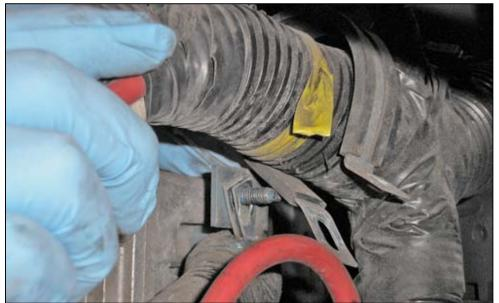
Rotate the clamp with the eyelet pointed up as shown. Secure with the stud nut and tighten to OEM spec.
