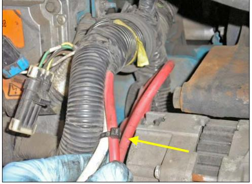
Carefully maneuver the cables toward the starter to allow sufficient length for proper connection to the B+ (30) terminal.
