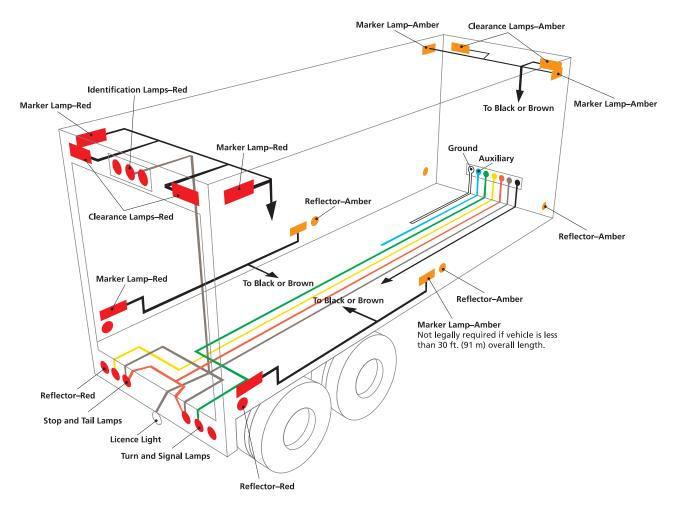
ATA. SAE & TTMA Wire Colours For Seven Pole Connectors
