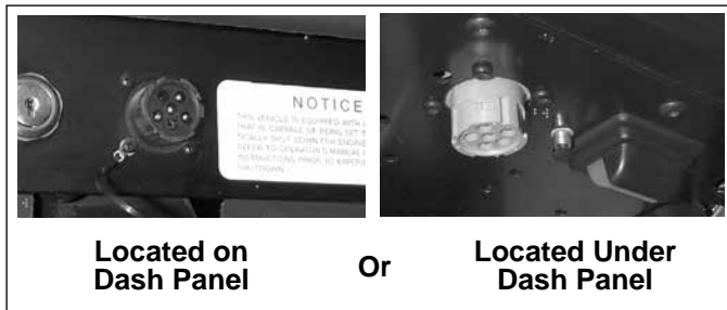
FIGURE 9 - TYPICAL VEHICLE DIAGNOSTIC CONNECTOR LOCATIONS (J1708/J1587, J1939)
