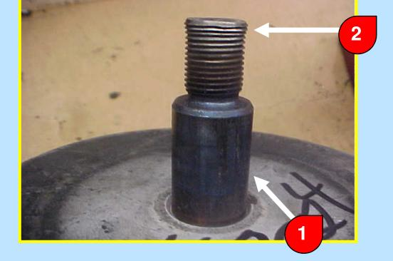
1- Pulley nut insufficiently tightened (blued shaft) as a result of improper installation, and/or insufficient vehicle maintenance.
