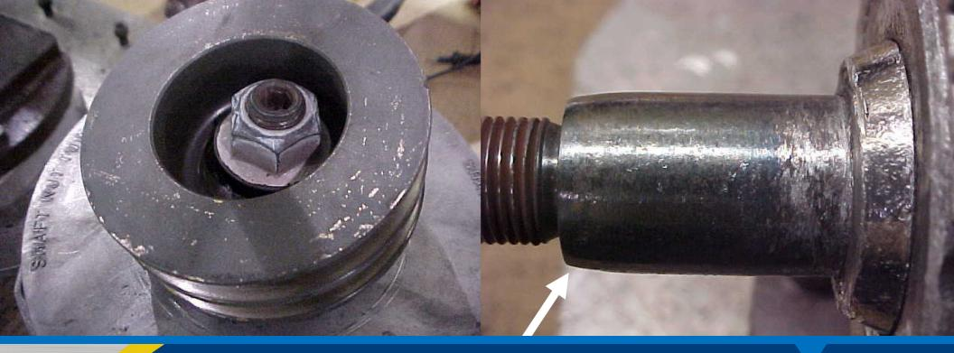
Pulley nut insufficiently tightened causing excessive wear on rotor shaft as a result of improper installation, and/or insufficient vehicle maintenance.
