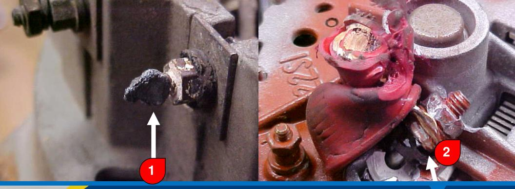
1- Terminal damaged due to heavy harness wiring arcing as a result of loose connection.
