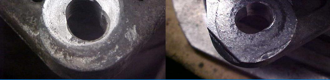
Physical damage to the product as a result of improper installation, and/or insufficient preventative maintenance – improperly tightened mounting bolt causing damage to alternator frame.
